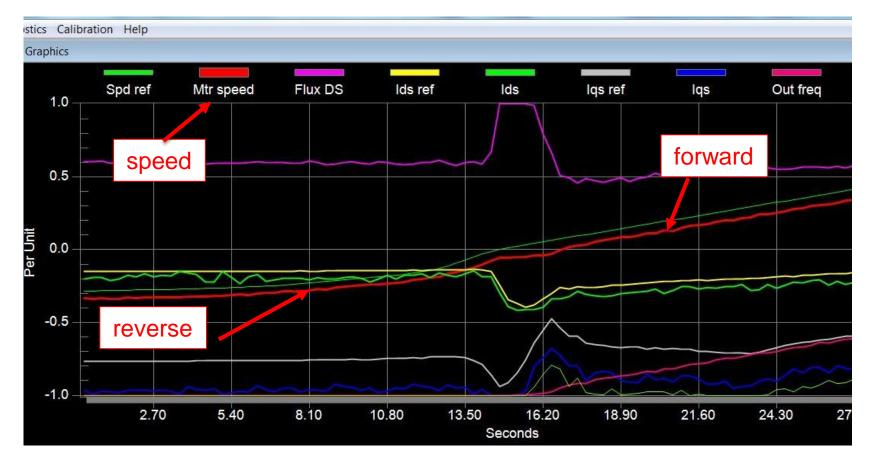
Catching a back-spinning load minimizes loss of production
