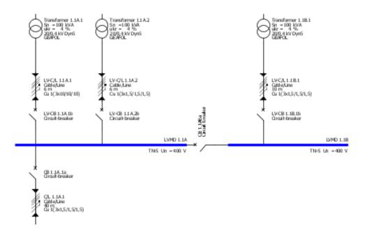
Now you can add distribution boards and load circuits to the new busbar for the new feed-in system linked by the coupling in the usual way.
