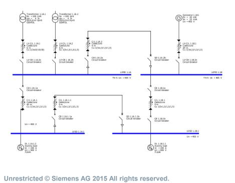
The diagram shows a network designed with one unidirectional coupling each at the main and sub-distribution board level.
