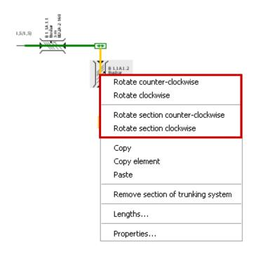
You can also adjust the graphical layout of busbars by calling up the corresponding functions for rotating the marked section, or rotating the entire busbar layout, from the context menu with a right mouse click.
