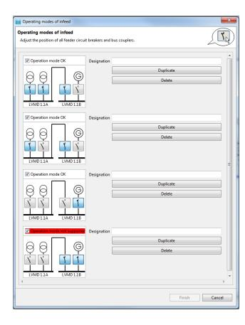
More operating modes are defined by duplicating the existing operating mode. Afterwards the switch positions are defined according to the new operating mode requirements.
