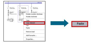
...then left-click to place it in the desired circuit as a substitute for the previously displayed item. Suitable elements on the network diagram that can be replaced are marked by a yellow frame upon mouseover.
