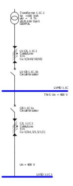
In principle, other distribution boards are created in the same way. A detailed description on how to add busbar trunking systems can be found in the "Busbar systems and loads" section.
