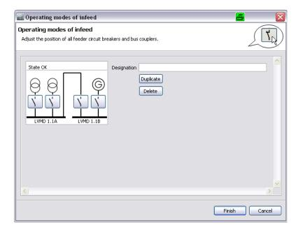
At first, only the structure of the configured infeed system is displayed. The switch position required for this particular operating mode can still be set by clicking on the switch symbol (open – closed).
