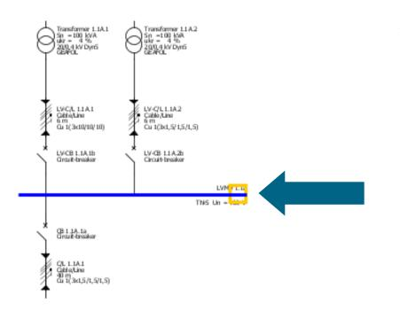
A "general coupling" is a coupling with an undefined direction of energy flow between busbar sections.
