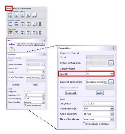
To simplify planning work for larger projects and maintain a straightforward structure of the network diagram, you can create **load groups**
