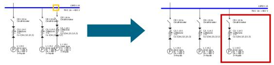
But individual elements of a circuit, such as a switching device or busbar section, can be copied and pasted to another circuit:
