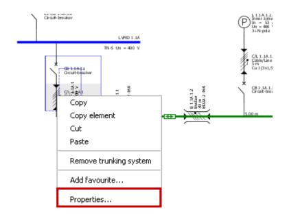
Another possibility is opening the "Properties" window by marking the element on the network diagram and selecting "Properties" from the context menu (right mouse button).
