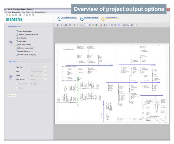
In the step "Project output", you can see the network diagram you designed on the right. It cannot be modified any more in this program step.
