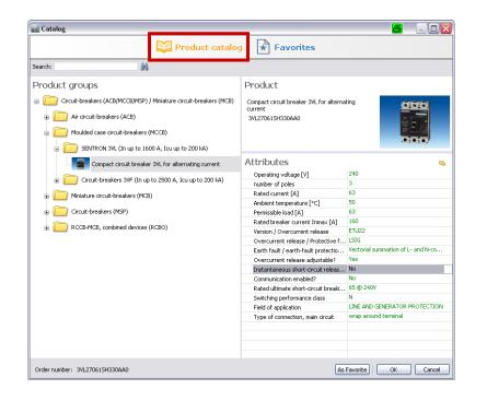
In the product catalogue, a specification is made based on the technical data that can be selected on the right.
