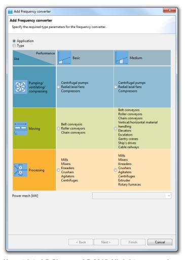
The type of **frequency converter** will be determined automatically by selection of classification, application and power.
