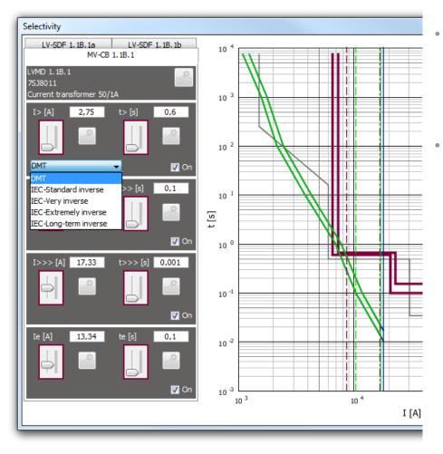
For medium-voltage circuit breakers you can select either DMT (Definite Minimum Time) or IDMT (Inverse Definite Minimum Time) in the selectivity window
