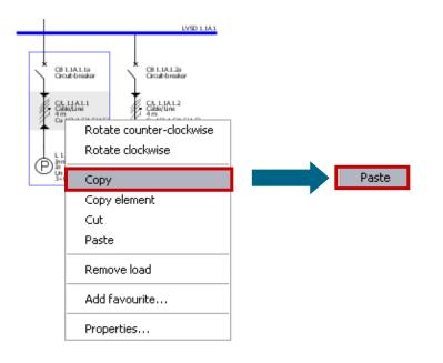
Please note that you have the option to copy entire circuits (e.g. load circuits or sub-distribution systems) and insert them at another position into the network by
