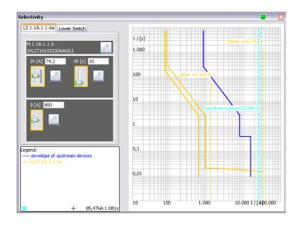
A window opens, where the current-time characteristic of the selected element as well as the envelope curves of the upstream and downstream device are displayed in a diagram.
