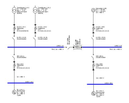
The possibility to dimension identical power sources connected in parallel and calculating the impact of this configuration on the short-circuit currents or load currents in the network, is extended by another option in **SIMARIS design professional**:
