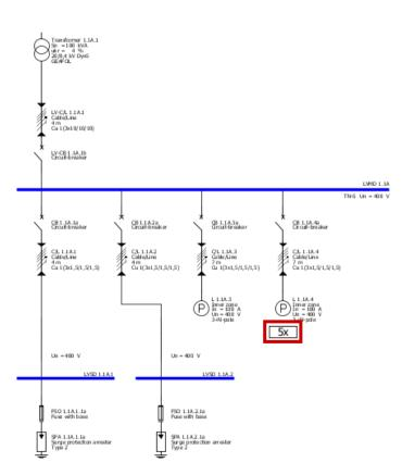
The selected number of identical loads is of course marked in the network diagram and automatically factored in during a subsequent dimensioning cycle.
