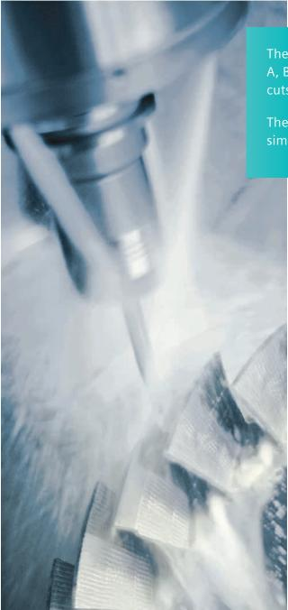
The three linear axes X, Y and Z and two rotary axes A, B or C are used for milling with aligned tools, relief cuts or geometries arbitrarily located in space.
