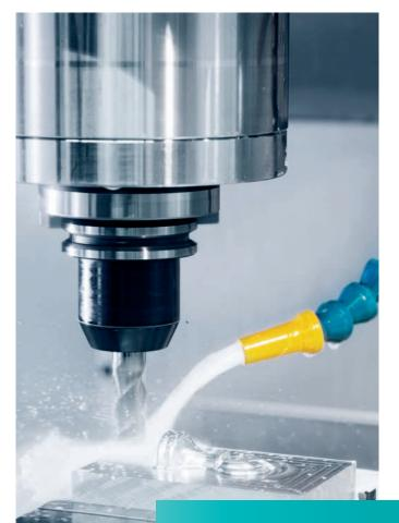
Top Surface optimizes CAM data for the subsequent path control leading to an even better surface finish. Advanced Surface has an optimized "Look ahead" algorithm, which leads to perfect surface quality with identical results in adjacent milling paths.
