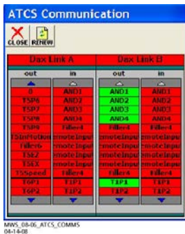
Figure 238: The ATCS Communications Window
