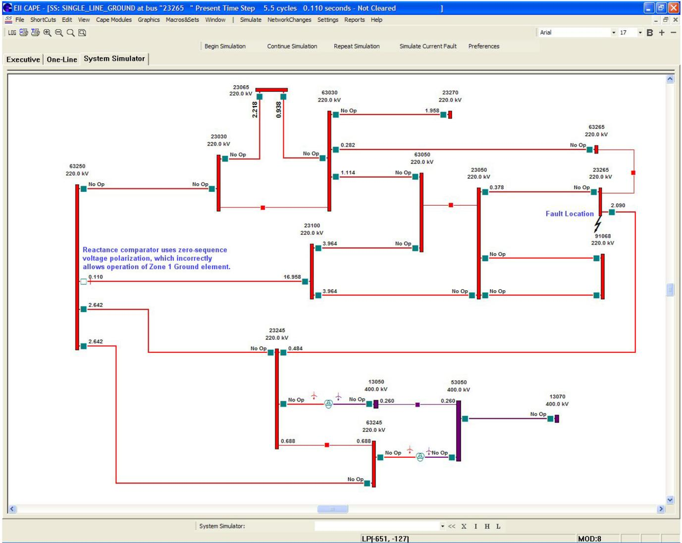
System Simulator's unique stepped-event simulation details every relay's response from the time you apply a fault until the last breaker opens to clear it. You do not have to tell it which devices provide primary protection.
