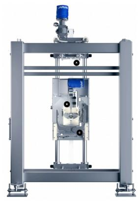
Three principal moving parts of the JLR-900 linear pork splitter: (A) leg spreaders to position the carcass for a precise cut; (B) stabilizing plastic rollers to align and totally control carcass movement; and (C) the body grabber that gently closes around the lower half of the carcass to further ensure a precise cut.
