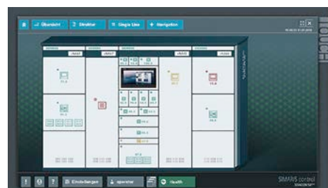
SIVACON S8 plus switchboard – Health Index
