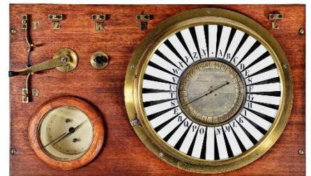
Werner von Siemens' electric pointer telegraph laid the foundation for a successful company's history.
