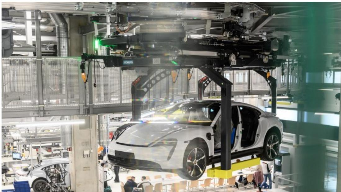
As, due to several building restrictions, the final assembly production line had to be built up vertically, a manufacturing concept has been developed in which each level is used for production purposes.
