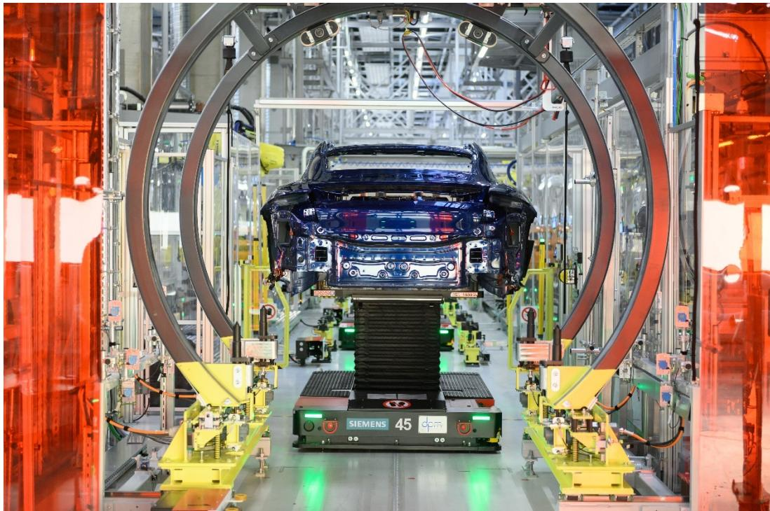
To ensure maximum flexibility in production, automated guided vehicles take the car bodies from one production station to the next.
