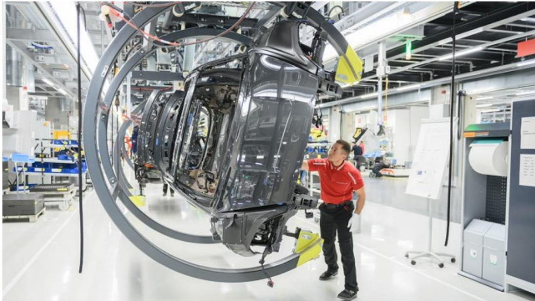
In addition to the automated guided vehicles and the door conveyor system, tilt EMS hangers are used to ensure ergonomic working conditions.
