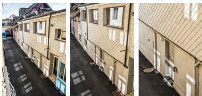
Fig. 7.2: Different fields of view: wide angle (left), normal (middle), telephoto (right)
