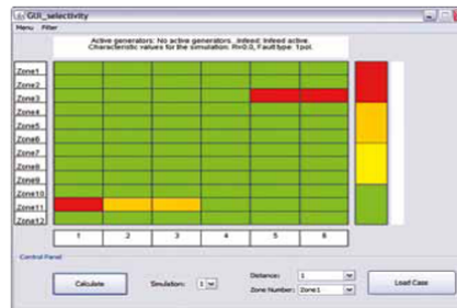
Figure 4: Evaluation of protection system performance with SIGUARD PSA
