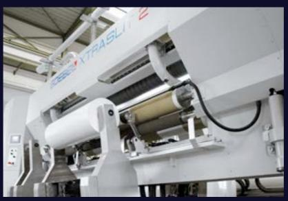
The GOEBEL XTRASLIT 2 is an innovative slitter rewinder and sets standards for highly productive processing of paper, film and foil, and flexible packaging materials.
