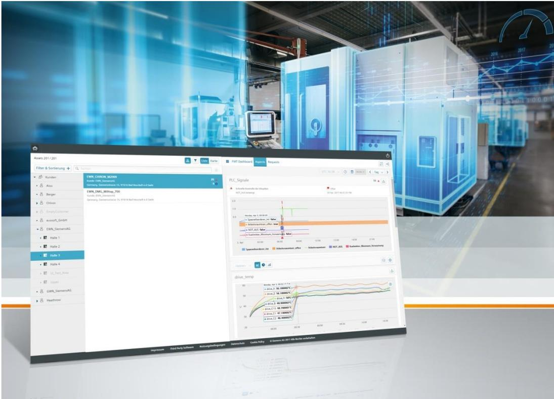
Manage MyMachines/Remote is a plug-in for the Manage MyMachines MindApp from Siemens which enables remote access to the CNC (Computerized Numerical Control), permitting complete remote control of the CNC by means of failsafe encrypted communication over the Internet.
