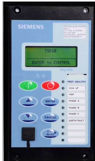
Figure 2-1 7SR10 Argus Overcurrent Relay with Control Push Buttons
