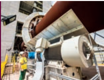
High efficiency main kiln-drive
