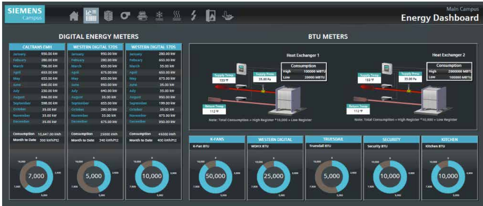
Automated energy consumption panel
