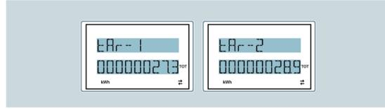
In addition to the total and partial energies, two independent tariffs can be managed for energy measurement.
