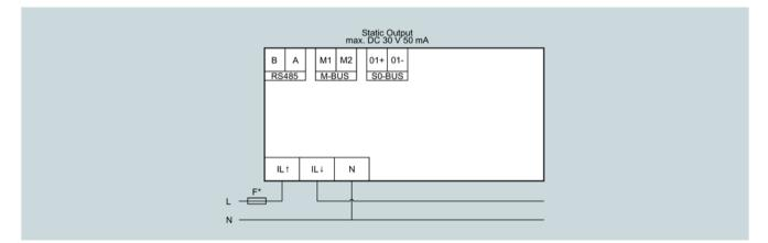
The fuse in the voltage measuring input is only used for cable protection.
