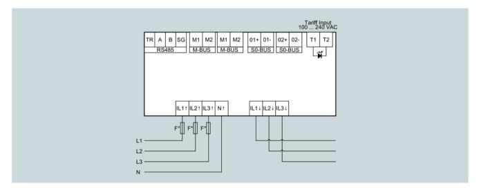
The fuse in the voltage measuring input is only used for cable protection.
