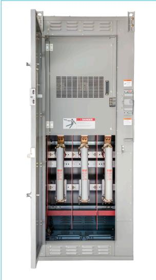
SIEBREAK metal-enclosed interrupter switchgear is of metal-enclosed construction as described in ANSI/IEEE standards. The equipment is tested and factory assembled in convenient shipping groups. It is ruggedly constructed of 11-gauge sheet steel including the doors. The assembly employs bolted construction.
