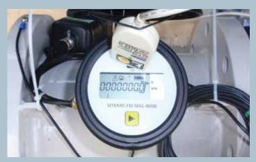
An infrared IrDA interface offers the ability to upload or download data via laptop.
