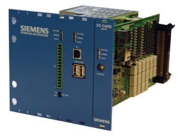
When used with Siemens controllers the interface between the equipments is via a simple serial link, reducing both installation and maintenance costs. In addition, reliability is enhanced as many physical terminations are avoided. Additional features such as remote access to the controller handset and complete upload and download of controller data are also offered.
