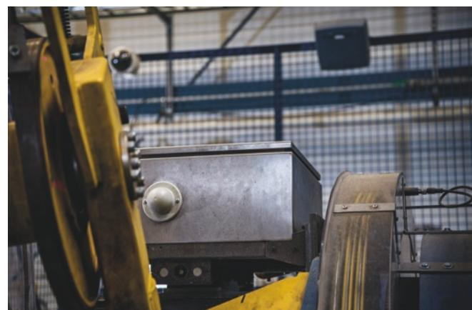
On the wall there is a SCALANCE W access point and ANT-795-6MN WLAN antennas are mounted on the rotation device opposite to one another. If the signal is lost for just 32 milliseconds, then the machine makes an immediate emergency stop.
