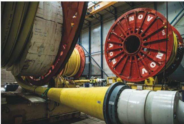
Some pipes are as long as 12-14 kilometers, and they are stored and transported around the plant on huge reels.
