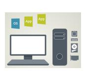
Through virtualization, the operating system and the user software of a computer are decoupled from its hardware.
