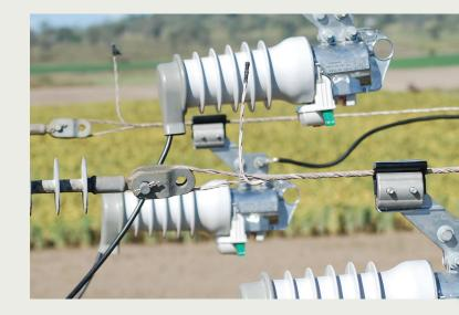
The small footprint and light weight of the Fusesaver™ enable quick and easy installation and fast commissioning. Self-powered from line current, the circuit breaker has the capability for multi-phase fault clearance for both transient and permanent faults. The smart system provides wireless connectivity for remote access and can be easily integrated into a utility's SCADA network via a Remote Control Unit (RCU).
