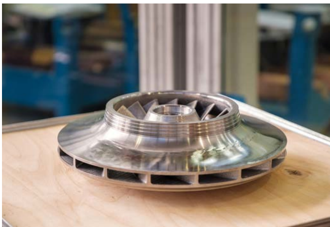
Figure 1. Additively manufactured radial impeller after overspeed test.
