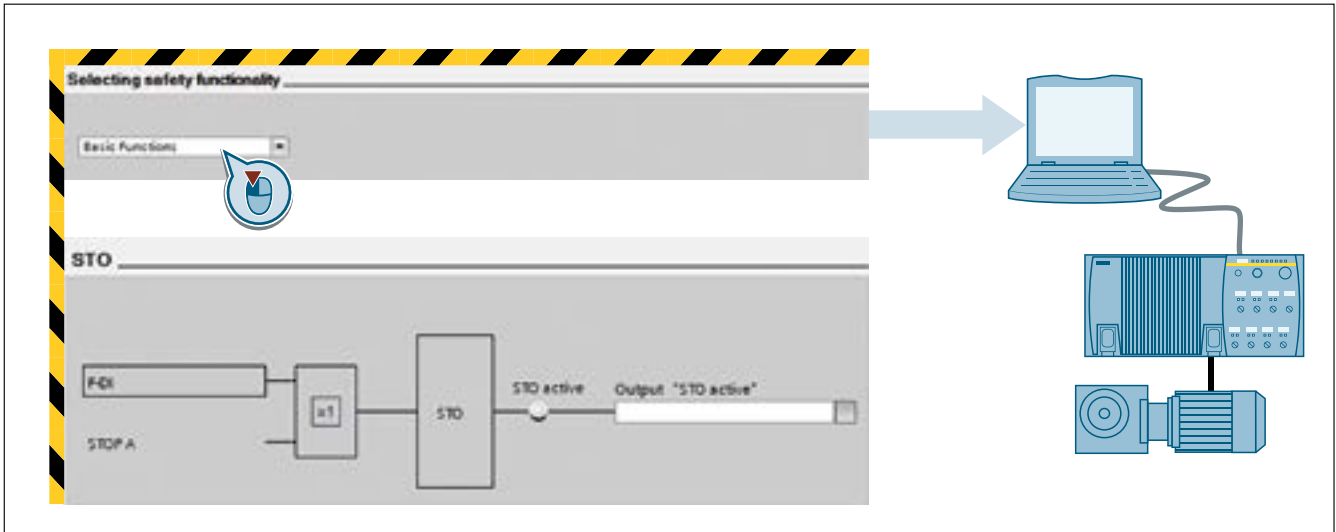
Figure 2-3 Commissioning the „Safe Torque Off“ (STO) function using Startdrive
