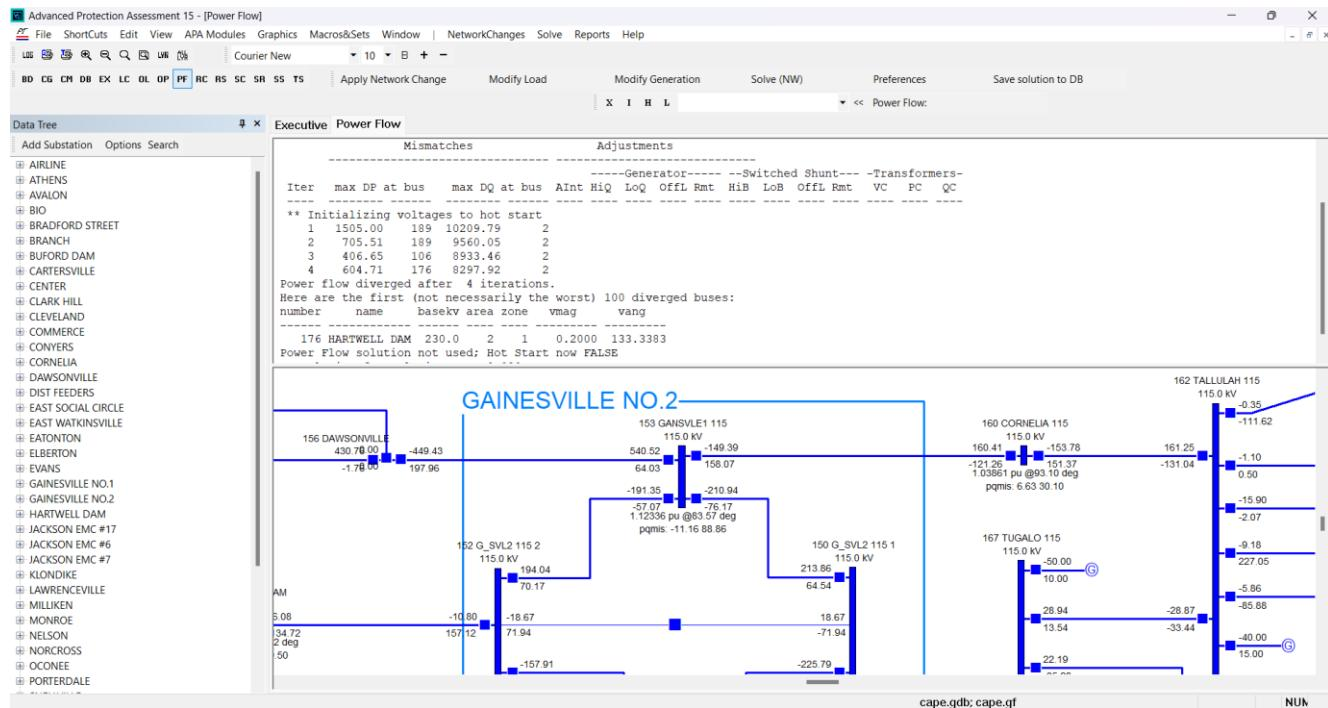
Figure 1: Power Flow gives you the two most effective algorithms available: Newton and Fast Decoupled. It gives you complete interactive control over the iterative solution procedure.
