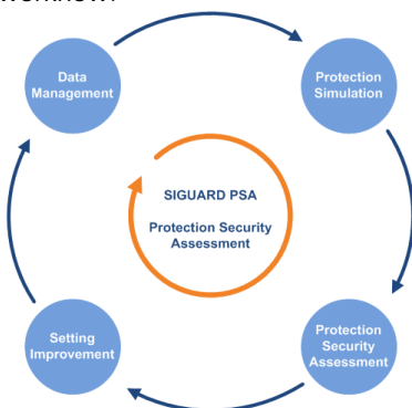
Figure 1: SIGUARD® PSA Workflow
