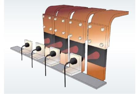
Installation example for IR temperature sensors for contact-free detection of the temperature development at the busbars
