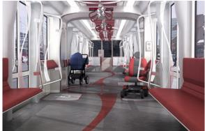
Other notable aspects of the S200 vehicles designed to increase passenger comfort and safety include slip-resistant flooring, on-board security systems, GPS mapping displays and larger windows and doors to increase natural light and provide visual security.
