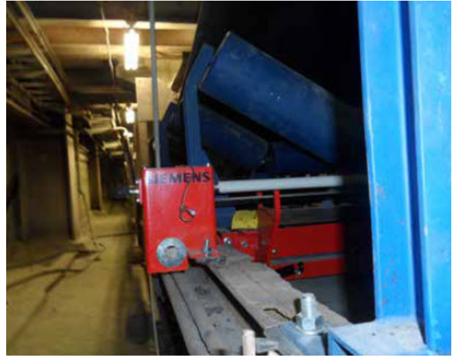
Milltronics BW500 is a full feature integrator for use with both belt scales and weighfeeders. Belt load and speed signals are processed for accurate flow rate and totalized weight of bulk solids.
