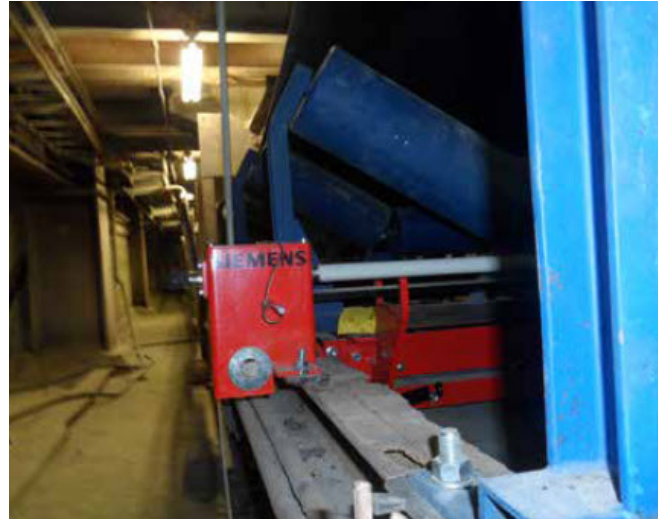
The Milltronics MWL weight lifter's modular construction easily adapts to different conveyor widths, including conveyors with belt widths as large as 96 inches.
