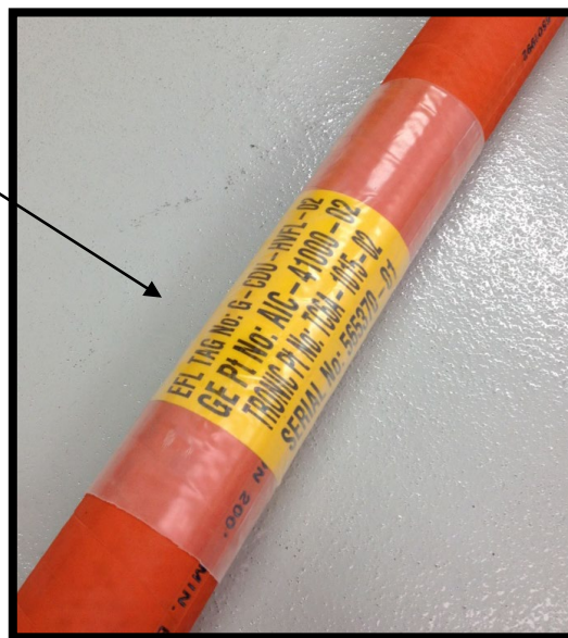
Figure 2 – Marking of Hoses
