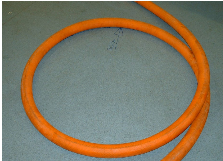
Figure 17-MBR being maintained (AquaTRON 200 Hose)
