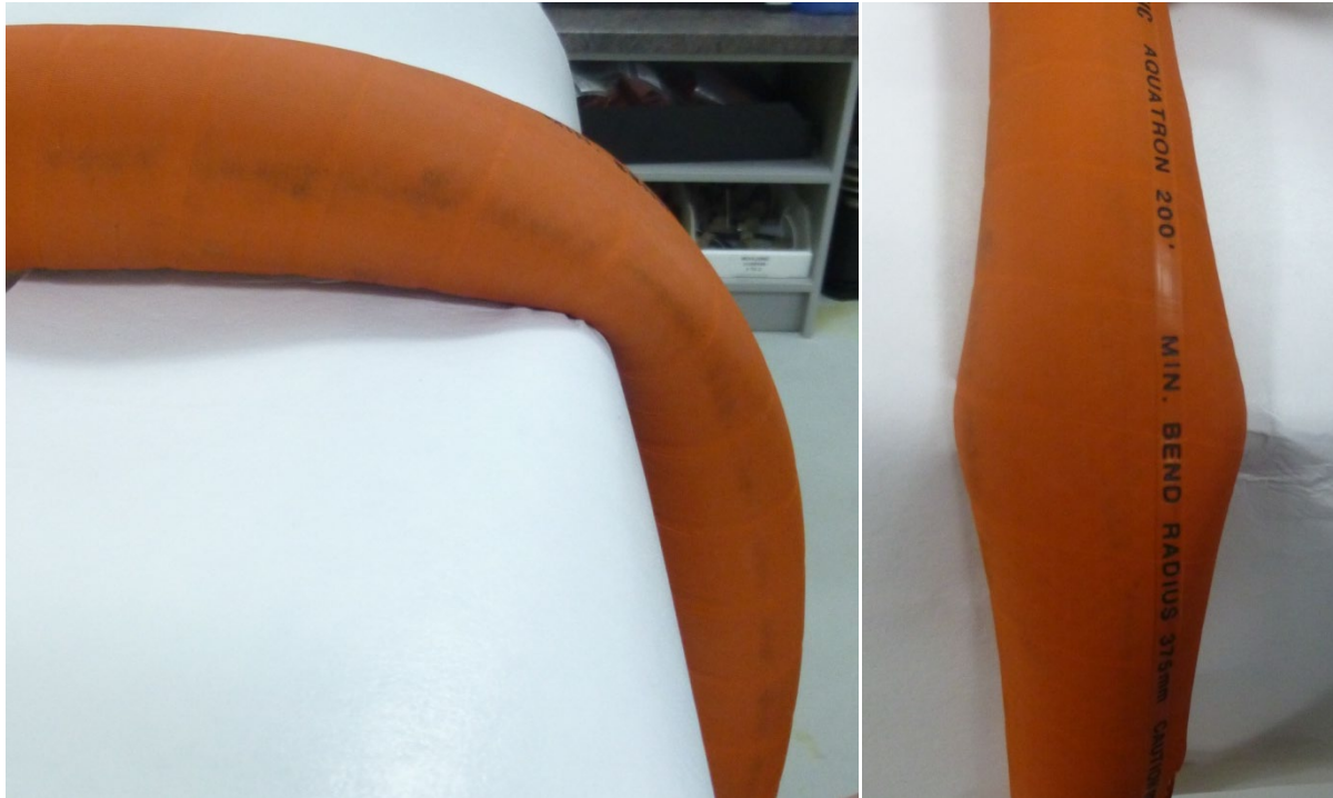
Figure 19-Incorrect routing (hose deformed over “sharp” edge- AquaTRON 200 Hose)
