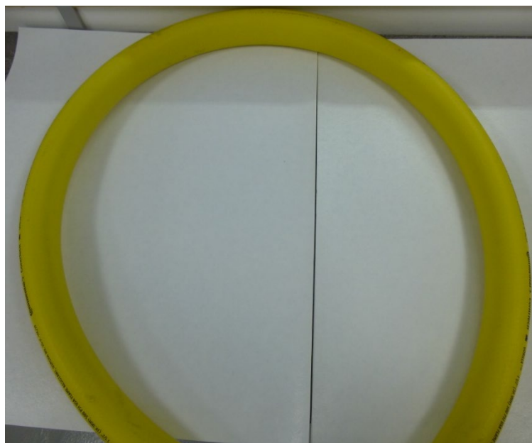
Figure 18- MBR being maintained (Gorilla 1.5" Hose)
