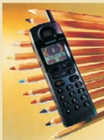
In the nineties, Siemens became involved in the development of mobile technology, which it later abandoned. Some of the usability solutions in Siemens mobile phones were new features – the S10 mobile phone from 1997 had a colour screen (with high-resolution for that time) and a button with a twenty second voice recording function.
