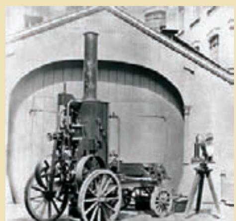
Mobilna »elektrarna« z žarometom, s kakršnim so najverjetne osvetlili Narodni dom, okoli 1873. A mobile power station with a headlamp such as the one that was most probably used to light up the National Centre, around 1873.
