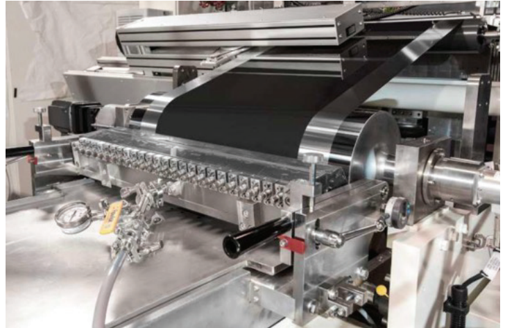
Figure 2. The GigaCoater coating station delivers the same quality top and bottom coating in a single pass with an ultra-precise \pm 1\% coating weight.
