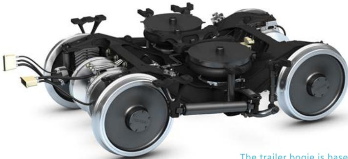
The trailer bogie is based on proven technology featured by the Desiro City: The short wheelbase – just 2,100 mm – and the very low weight of the new bogie design lead to significant improvements in energy consumption, track-friendliness, and wheel wear.
