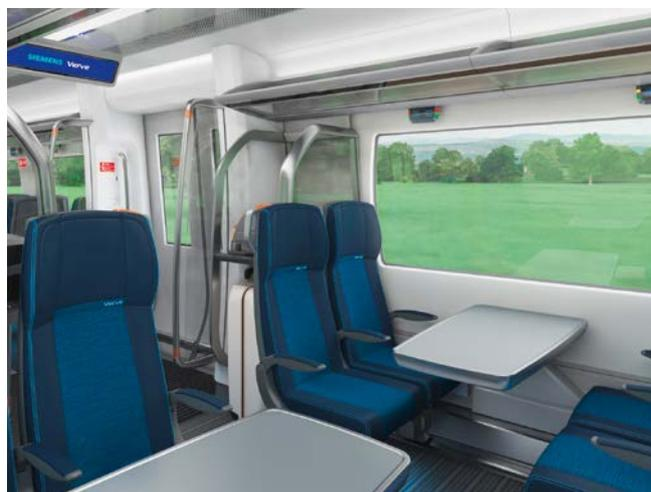
The seating has been designed taking ergonomics as well as additional space and passenger comfort for intercity travel into account. The standard seats have a slim visual aesthetic that lends a contemporary design appearance to the Standard Class saloon and creates a feeling of spaciousness in the vehicle.
