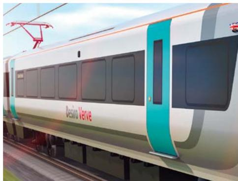
Desiro Verve can even be equipped with single-leaf end doors or double-leaf plug sliding doors at 1/3 – 2/3 position.
