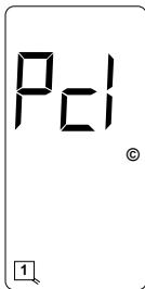
Loop Check Pending Indication
