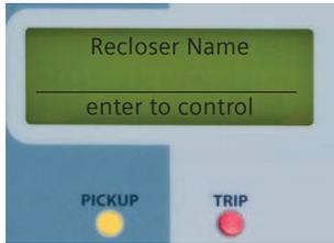
← If the LCD screen does not read ENTER to CONTROL, press
