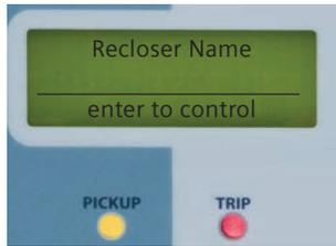
← If the LCD screen does not read ENTER to CONTROL, press
