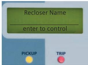
← If the LCD screen does not read ENTER to CONTROL, press
