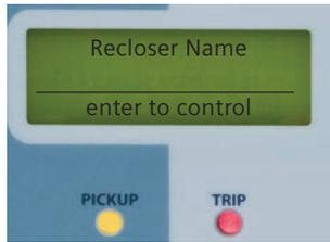
← If the LCD screen does not read ENTER to CONTROL, press
