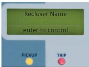
If the LCD screen does not read ENTER to CONTROL, press
