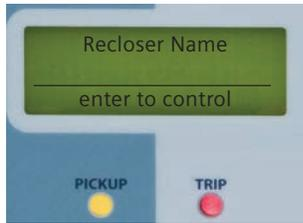
← If the LCD screen does not read ENTER to CONTROL, press
