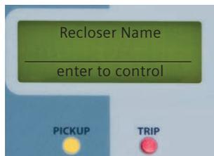
If the LCD screen does not read ENTER to CONTROL, press
