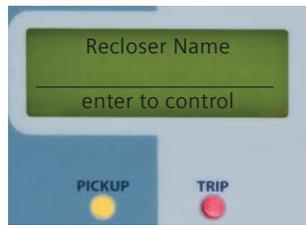
If the LCD screen does not read ENTER to CONTROL, press
