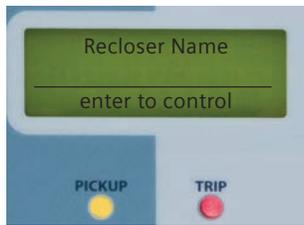
← If the LCD screen does not read ENTER to CONTROL, press
