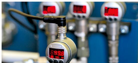
Monitoring elements of the hydraulic controller
