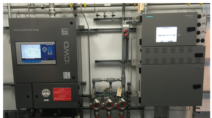
MAXUM II Process GC for Speciated Measurement and CWD2005 Calorimeter for continuous and fast on-line Heat Value Measurement
