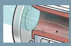
Minerals or particles will bounce off the soft rubber liner instead of wearing it down.
