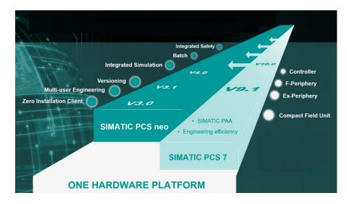
Siemens Supports Two DCS Software Lines that Share a Common Hardware Platform
