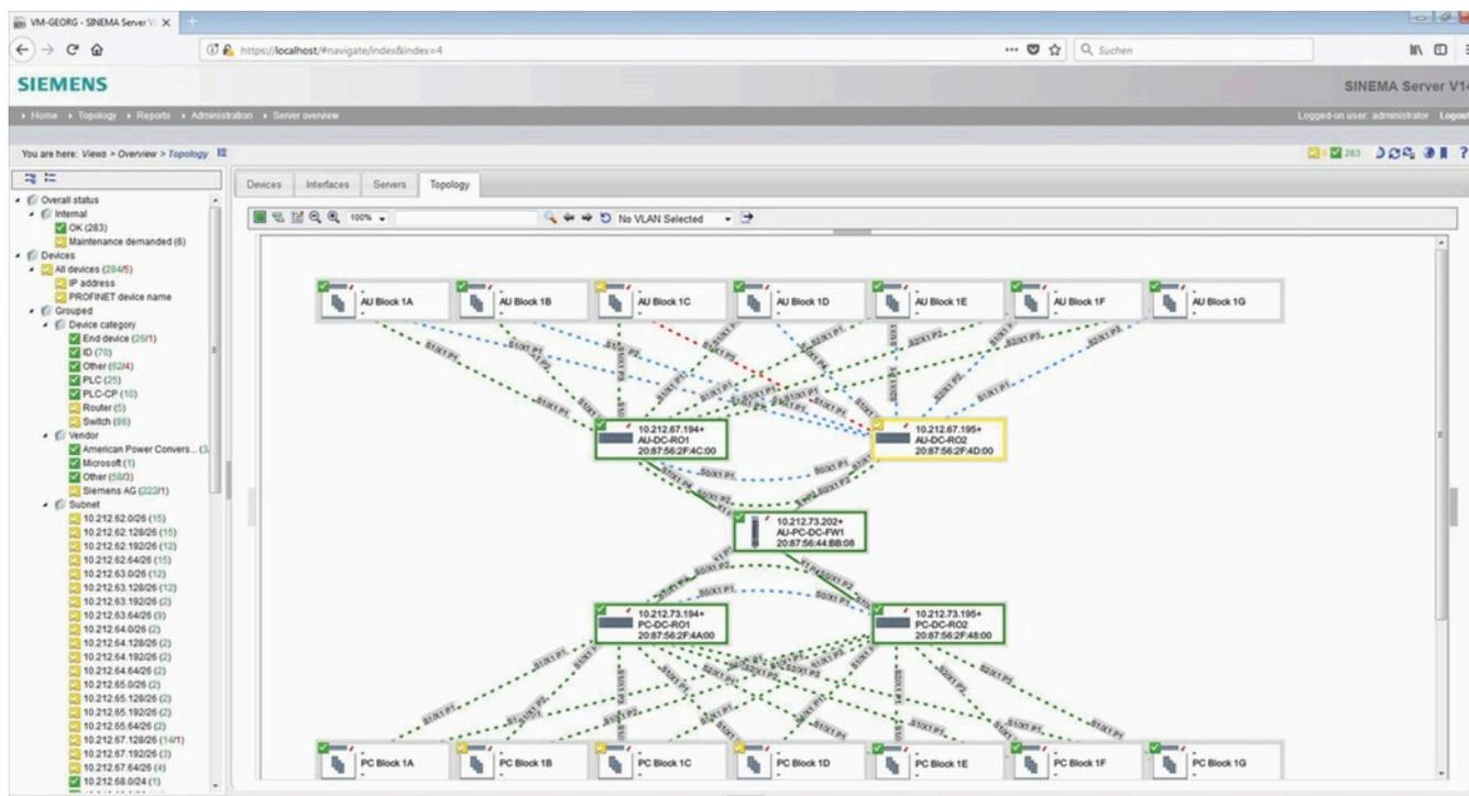
The network devices were successively commissioned from afar via the SINEMA Remote Connect management platform for remote networks. The entire network solution can be conveniently monitored from afar via the SINEMA Server network monitoring and diagnostics software (pictured).
