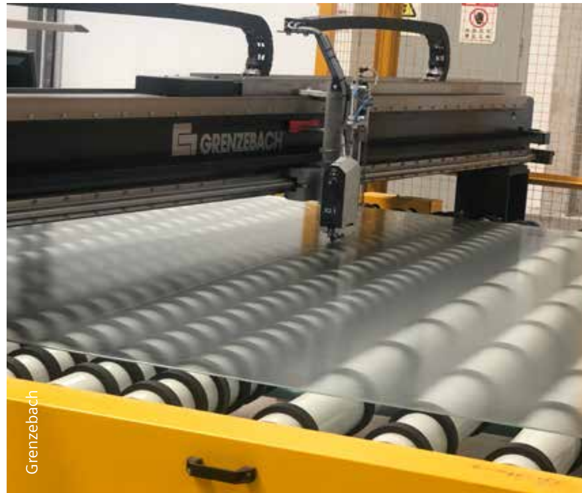
Cutting technology lies at the heart of the cold end of a flat glass production line and plays a decisive role in efficiency and running time. With Simatic AX, Grenzebach and Siemens are driving the transition to an advanced, IT-oriented engineering ecosystem.
