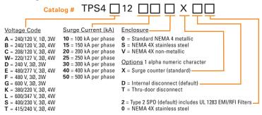
Example: **TPS4C12200XD2** = a Type 2 SPD for a 208/120V application with a surge current capacity of 200kA per phase, in a standard NEMA 4 enclosure with a surge counter and internal rotary disconnect option.
