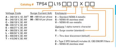
Example: TPS4CL15900XT2 = a Type 2 SPD for a 208/120V application with a surge current capacity of 900kA per phase, in a standard NEMA 4 enclosure with a surge counter and thrudour disconnect.
