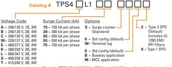
Example: TPS4CL120X000 = SPD for a 208/120V panelboard with a surge current capacity of 200kA per phase and a surge counter option.
