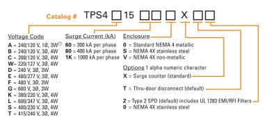
Example: TPS4C15800XT2 = a Type 2 SPD for a 208/120V application with a surge current capacity of 800kA per phase, in a standard NEMA 4 enclosure with a surge counter and thrudour disconnect
