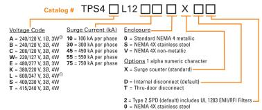
Example: **TPS4CL12300XT2** = a Type 2 SPD for a 208/120V application with a surge current capacity of 300kA per phase, in a standard NEMA 4 enclosure with a surge counter and thrudoor disconnect.
