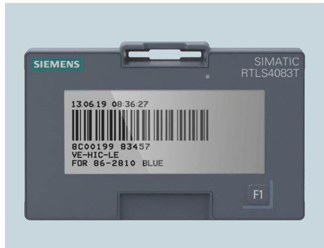
Several thousands of these new, approximately credit-card-sized transponders – SIMATIC RTLS4083T with 2.7" e-ink display and rechargeable battery – make the automotive pre-assembly and final assembly efficient and process-reliable.
