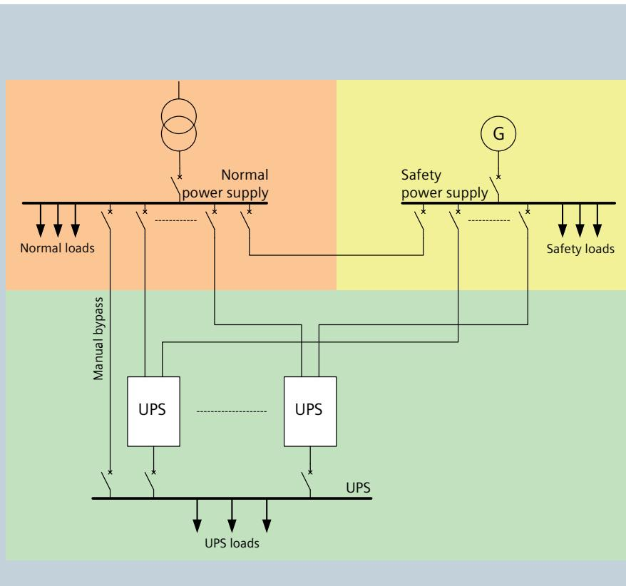
*Fig. 2: Supply of a short circuit on the output side by the transformer through the bypass or/and through the inverter*
