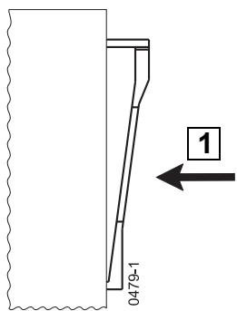
**Installing display and latching it tight**
