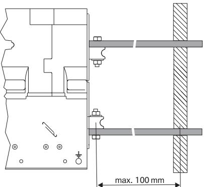
**FS III breaking capacity C ( $I_{cs} = I_{cu} > 100 \text{ kA}$ )**
