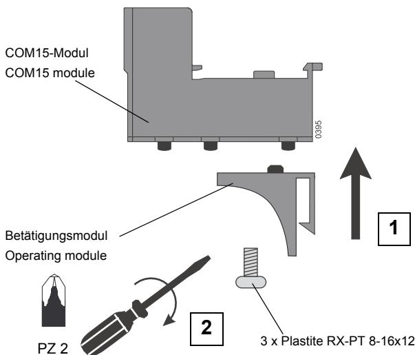
**Fitting COM15 module on the fixed-mounted breaker**
