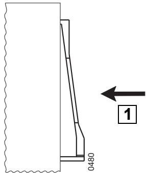
Installing the display turned by 180° and latching it tight
