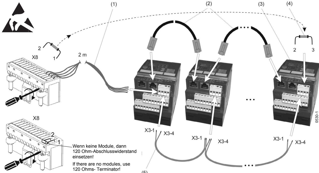
Only one **CubicleBUS**-module can be connected directly to a circuit breaker. Further modules must be connected from module to module. Spur lines are not permissible!
