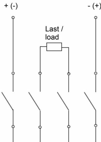
geerdete Photovoltaikanlage / electrical grounded application
