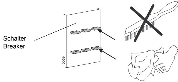
**Cleaning the main conductor connection**
