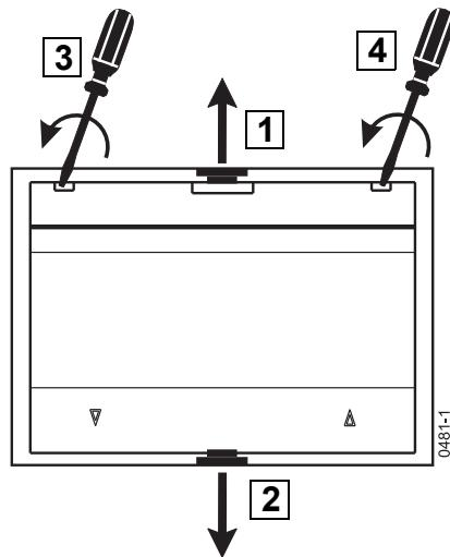
**Removing dummy flange**
