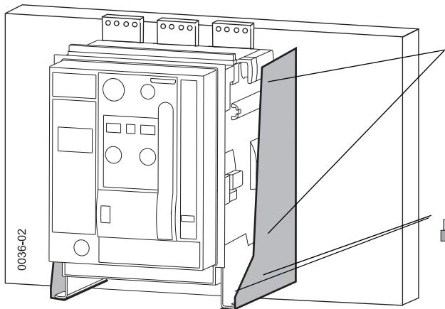
If several draw-out circuit breakers are arranged one above the other in cubicles **without** compartment bases we recommend to use arc chute covers.
