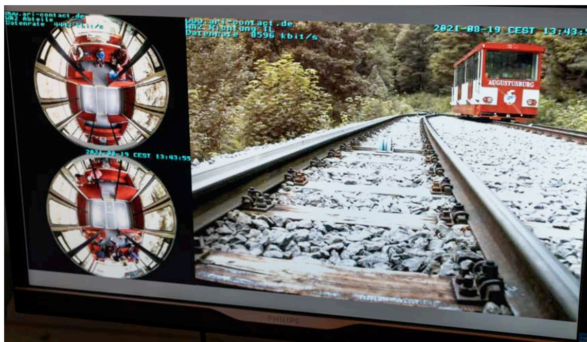
High-definition video footage of the track and the car's interior are transmitted via the IWLAN network.
