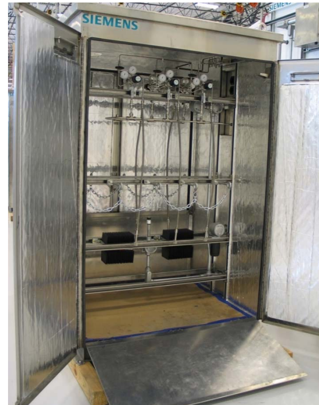
Heated Cabinet for Calibration/Validation
