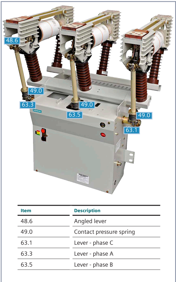
Figure 6: Vacuum circuit breaker magnetic-actuator operator module
